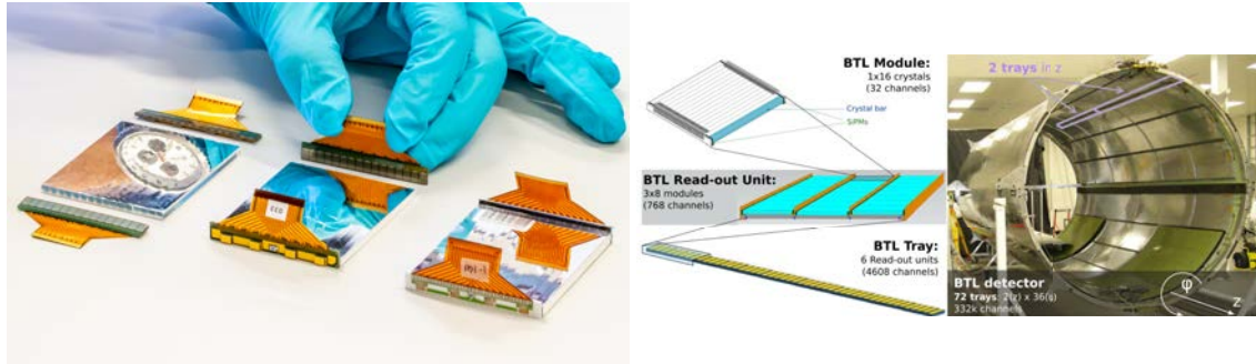
Figure 2: Left: Picture of BTL sensor modules. Right: Hierarchical structure of the BTL components (left) and trays enclosed within the mechanical support (right).
