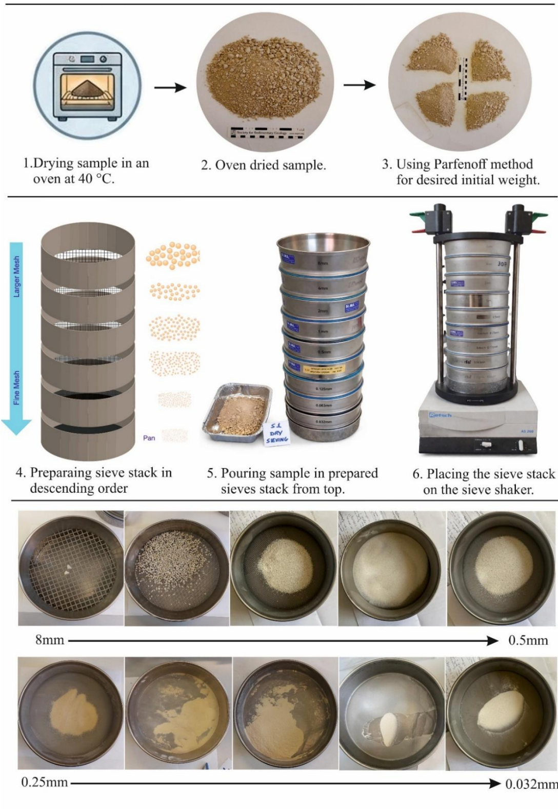
Figure 2.5 The figure illustrates the sequential steps involved in determining the grain size distribution of the sand sample. Following oven drying, a representative sample was accurately weighed and prepared for analysis (first row). The second row shows the arrangement of a standard sieve stack in descending mesh size. The third row presents the individual sieves after sieving, each containing the fraction of particles retained according to size.
