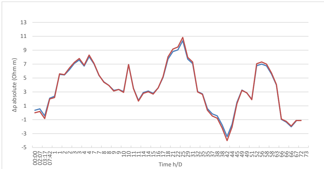
Figure 5.1.1 – Comparison between original \Delta\rho_a (red line) and temperature-corrected values (blue line), confirming minimal thermal bias.
