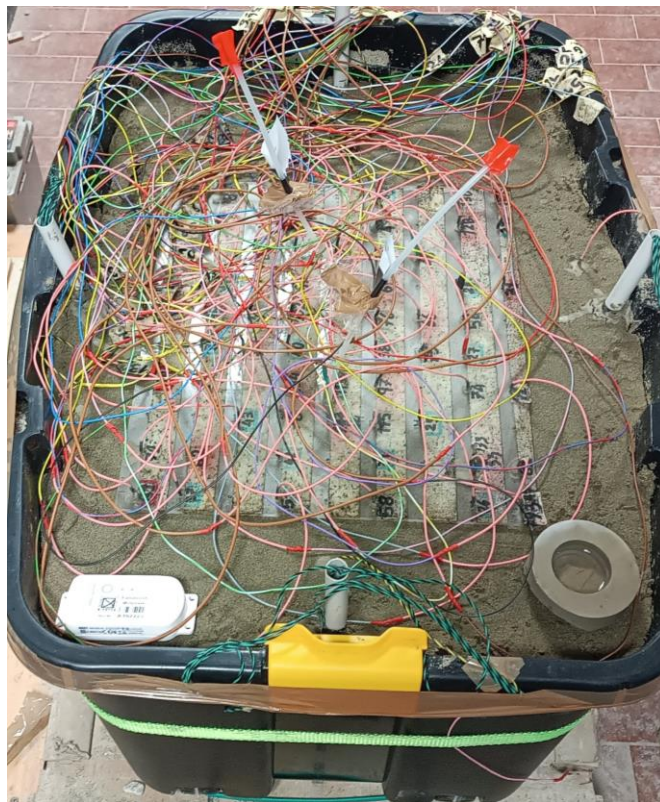
Figure 3.7.a – Location of HOBO sensors for environmental monitoring and corresponding temperature trends. Modified from experimental data (2025).
