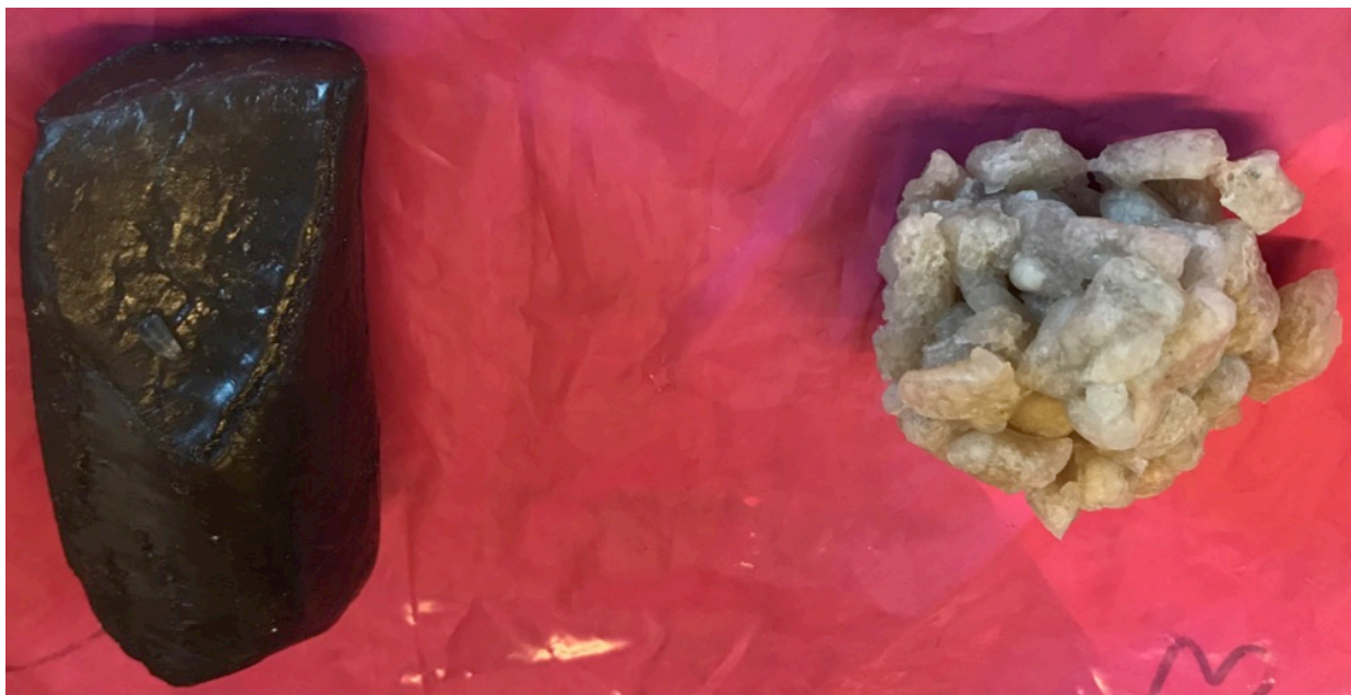
FIGURE 34 - A) SAMPLE OF COMMERCIAL SKI3 IR BEFORE PURIFICATION. B) SAMPLE OF PURIFIED IR.
