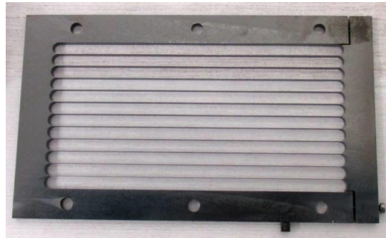
87 88 Figure 2: Example of the 3 mm thick grids used in the converter after ^{10}\text{B}_4\text{C} coating. The 89 thickness of thin walls is 200 \mu\text{m} . The external area of the grid is 12 cm x 7 cm; the frame 90 surrounding the thin walls is 1 cm thick.
