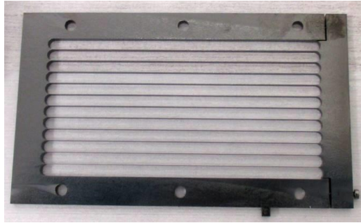
Figure 2-46: One of the 3 mm thick grids used for the production of the 3D-C after ^{10}\text{B}_4\text{C} coating. The thin walls are 200 \mu\text{m} thick
