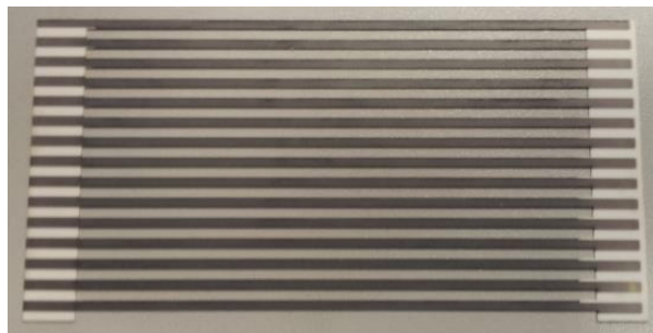
Figure 2-17: \text{Al}_2\text{O}_3 lamella coated with 1\ \mu\text{m} of ^{10}\text{B}_4\text{C} along the strips.
