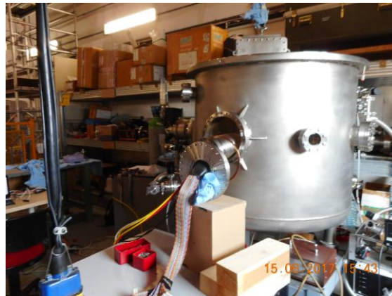
Figure 3-49: Installation of the detector box in the vacuum chamber
