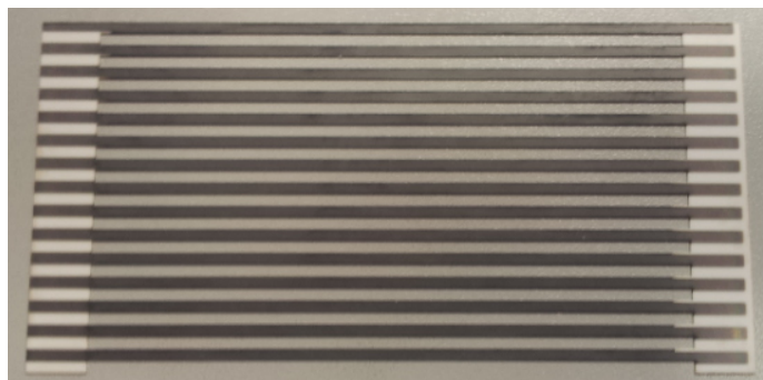
Figure 1. Coated \text{Al}_2\text{O}_3 lamella.
