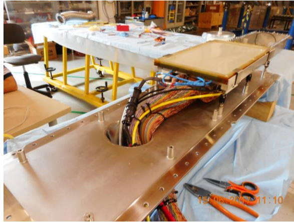
Figure 3-46: The nGEM detector installed on the detector box lid.
