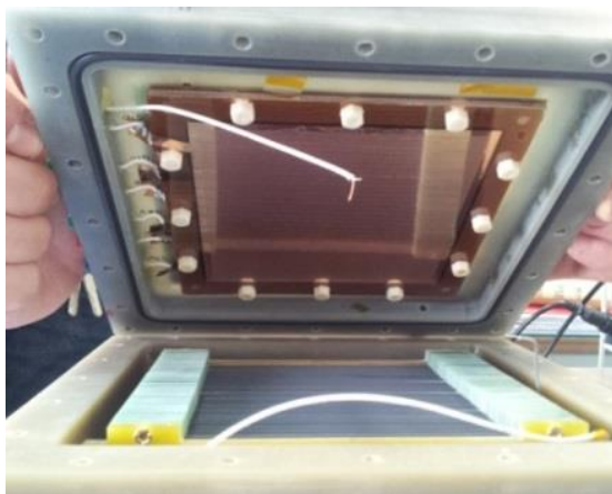
Figure 2-21: Coupling of the lamellas box with the triple-GEM box.
