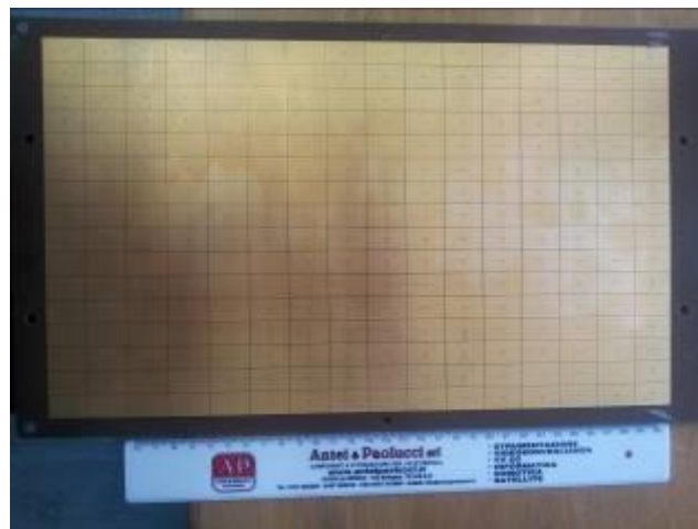
Figure 3-17: The padded readout anode of the nGEM detector
