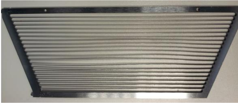
Figure 2-115: Grid realized with the design of the simulation reported in Figure 2-110. The bending of the strips is not acceptable.
