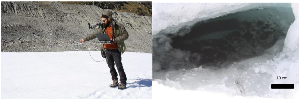
Figure 2 Left: Reflectance measurements during the second campaign (30 th September) at Morteratsch glacier. Right: An example of cryoconite hole found on the ablation area of Morteratsch glacier (Photos by R. Garzonio.)
