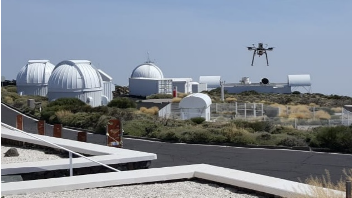
Figure 4. Photograph of the telescope and the UAV during the landing phase, taken near the home location. The black baffle of the second QUIJOTE telescope (the one on the right) is clearly visible beneath the UAV. The first QUIJOTE telescope is parked, pointing to zenith in the image.
