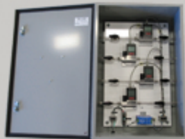
Gas Mixing System
