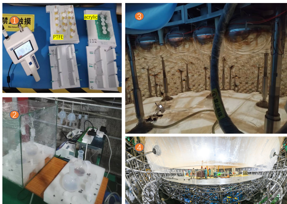
Fig. 4 Some sampling pictures in JUNO experimental hall. 1 and 2 depict the sampling photographs taken from the installation room and the hall floor, respectively. 3 shows the sampling image captured between the layers of acrylic sphere and the PMTs. 4 illustrates the installation platform for the acrylic sphere, where we conducted our sampling
