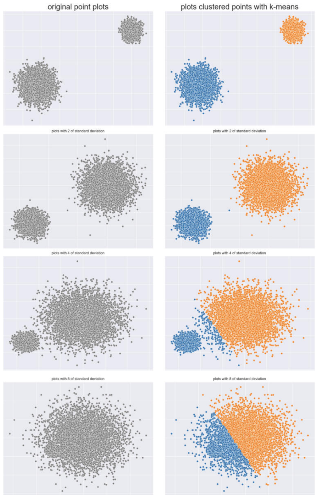
Figure 7 Two balls original dataset (left) and results obtained by k -means (right).
