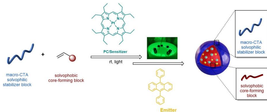
Scheme 4.2: Schematic representation of the one-pot production of UC polymeric nanoparticles via PET-RAFT polymerization.
