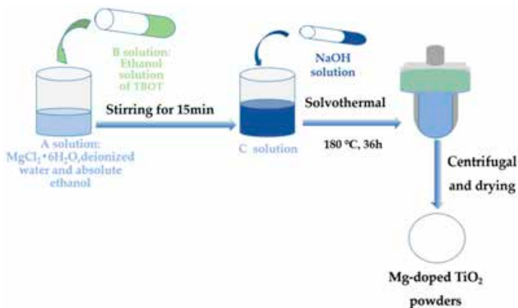
Figure 1. Schematic diagram of Mg-doped \text{TiO}_2 sample preparation.
