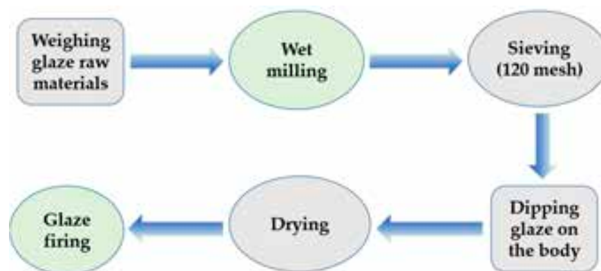
Figure 2. Schematic diagram of the glaze firing processes.
