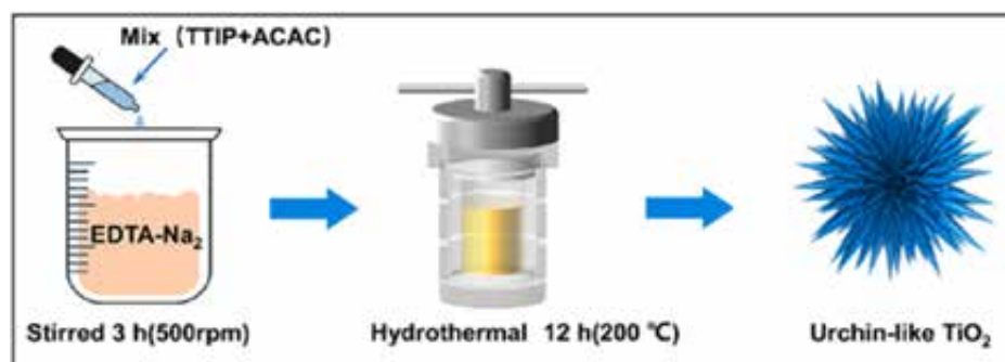
Figure 4. Preparation process of sea urchin-type titanium dioxide [47].
