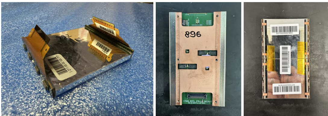
Figure 5.60: Each detector module is assembled from two pre-assembled and qualified sensor modules, which are subsequently connected to the front-end and inserted into the copper housing. A picture of a sensor module and of the two sides of a detector module are shown from left to right, respectively.
