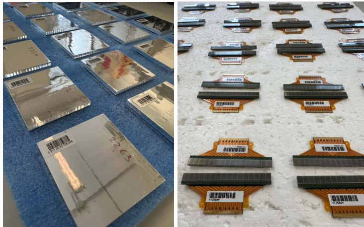
Figure 5.56: Pictures of LYSO:Ce crystals (left) and SiPM arrays (right) used for production at the Milano-Bicocca assembly center.
