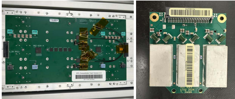
Figure 5.48: Left: A picture of a production CC mounted on a cold plate is shown. The connectors for cables providing TEC power, board power, and chip biasing (colored connectors) are visible. The fibers to be connected for readout via Serenity are protected with Kapton tape before connection, and the connectors on the sides, where the PCCs will later be attached, are also visible. Right: A picture of a PCC is reported.
