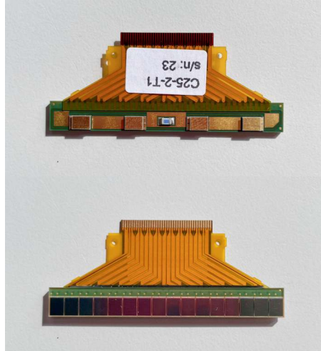
Figure 5.7: A picture of both sides of the SiPM array is shown: the back side, where the four TECs and the RTD are visible, and the front side, showing the active area of the 16 SiPMs at the bottom.
