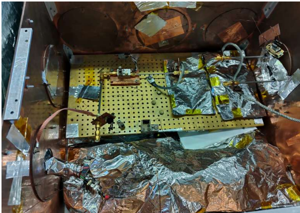
Figure 5.14: LNA setup to measure its noise temperature.
