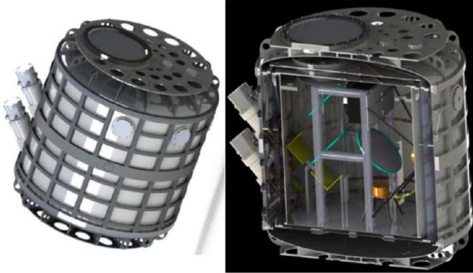
Figure 2.10: 3D rendering of the COSMO cryogenic system.
