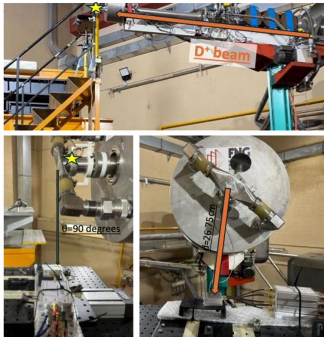
Figure 4.6: Experimental set-up at the FNG DT neutron source, for the characterization of the D4N diamond matrix.
