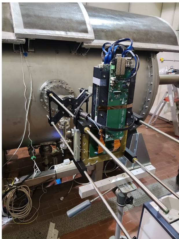
FIGURE 5 Picture of the gas electron multiplier detector installation.
