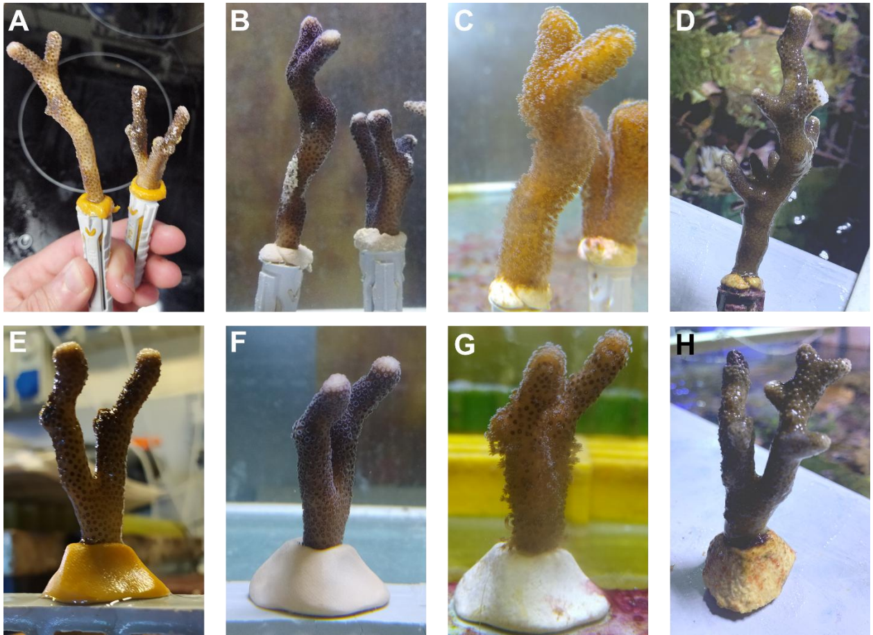
Figure 10. Coral putty in aquarium. A-D) Photographs of a Stylophora pistillata nubbin fixed with the coral putty inside a dowel Fischer as support immediately after the application and at 0, 30, and 90 days, respectively; E-H) Photographs of a Stylophora pistillata nubbin fixed directly with the coral putty without support immediately after the application, and at 0, 30, and 90 days, respectively. In both cases, 4 grams of coral putty were used, and the nubbins were inserted around 2 cm into the putty.
