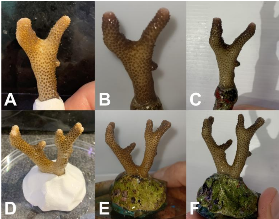
Figure 12. Aquamend in aquarium. A-C) Photographs of a Stylophora pistillata nubbin fixed with the Aquamend inside a dowel Fischer as support after 0, 30, and 90 days, respectively; D-F) Photographs of a Stylophora pistillata nubbin fixed with Aquamend as support after 0, 30, and 90 days, respectively.
