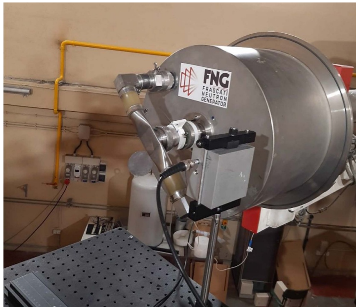
Figure 3. The SiC100 inside its aluminum casing installed on the FNG neutron source during the DT campaign. The 90^\circ angle ensured that the neutrons reaching the detector had energy E_n = 14.06\text{ MeV} .
