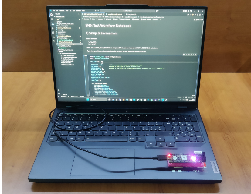
Figure 4.1: Experimental Validation Setup. The FPGA development board is connected via UART to the host PC, where a Python environment performs real-time data injection and results analysis.
