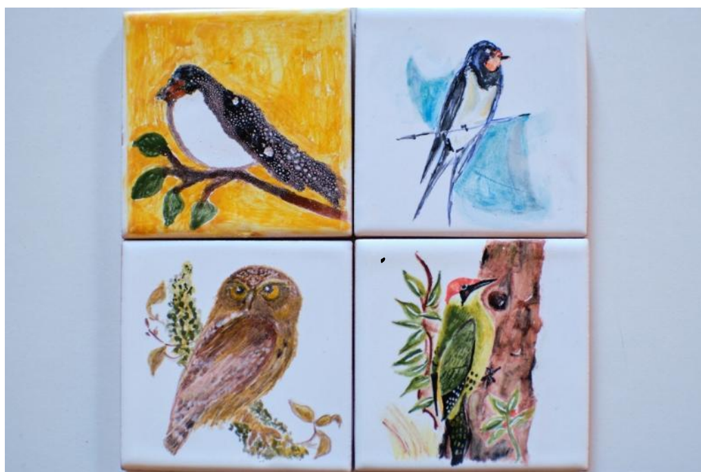
Figure 31: Examples of painted tiles after firing. The upper left tile shows how overhydration of the glazing surface during painting reacts during the firing, displaying a pitted effect on the surface. (03.07.2023).
