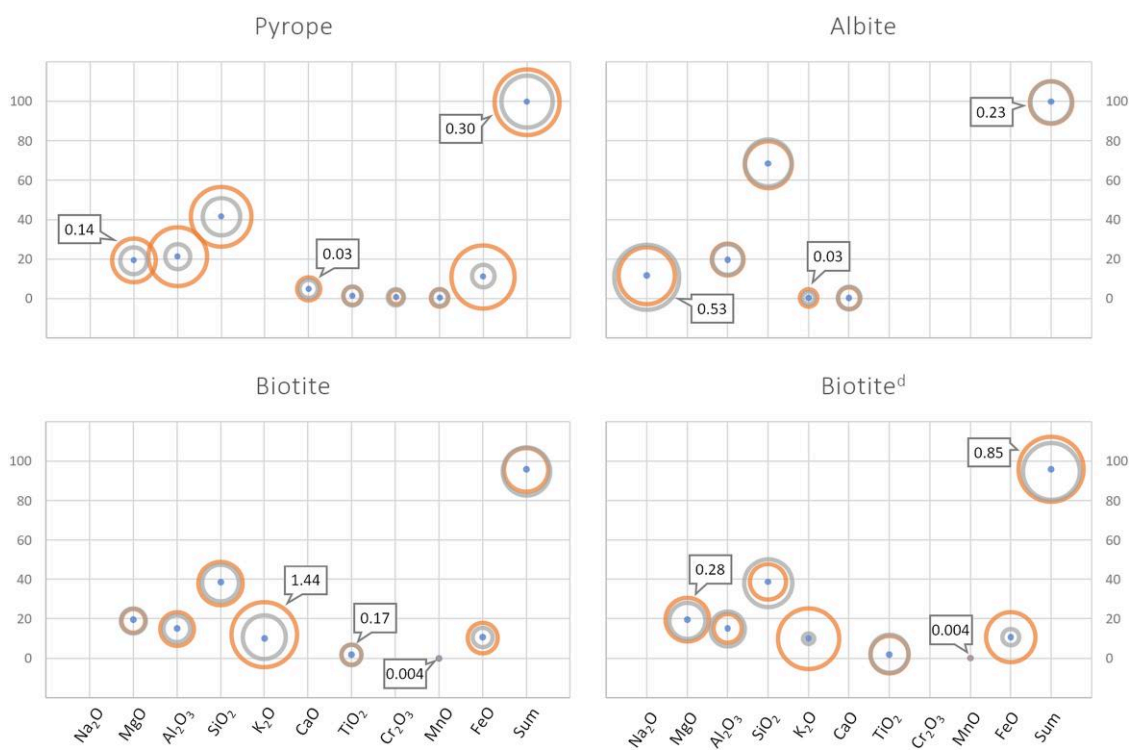
Fig. 4. Synoptic representation of the reproducibility of the measurements plotting the standard deviations reported in Table 1 for WEDS (orange) and EDS (gray): pyrope (upper left), albite (upper right), biotite (lower left), and biotite analyzed with defocused beam (lower right). Bubbles are centered on the average value of the relative oxide and their area is proportional to the standard deviation (some values labeled as size guide). The point at the center of the bubbles represents the nominal composition of the standard.
