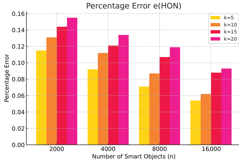
Figure 3. Percentage error e(HON) for different values of number of smart IoT objects n and number of groups k .
