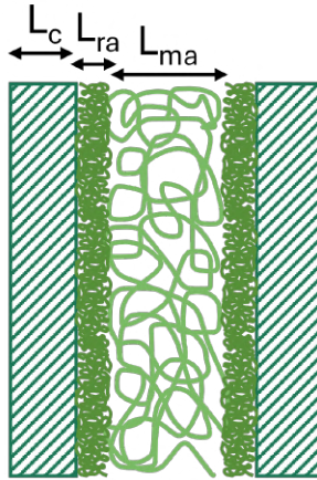
Figure 2.5: Scheme of the lamellar morphology of PLLA using the three-phase model: the crystalline layer ( L_c ), the rigid amorphous fraction (RAF) ( L_{ra} ), and the mobile amorphous phase ( L_{ma} ) [97].
