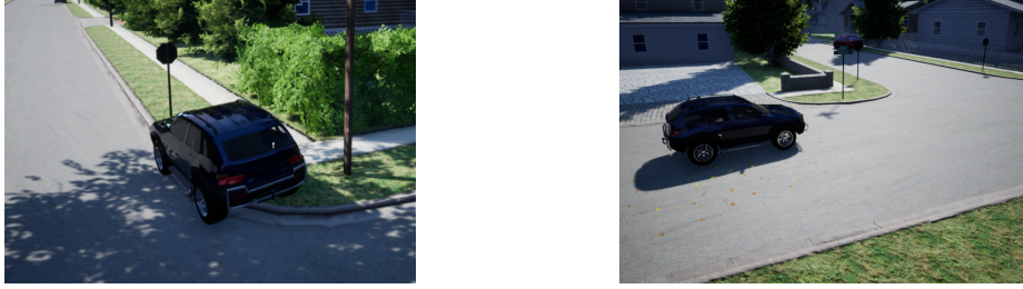
Fig. 4. AirSim Neighborhood simulation environment. Left: obstacle avoidance scenario. Right: left-turn navigation scenario.
