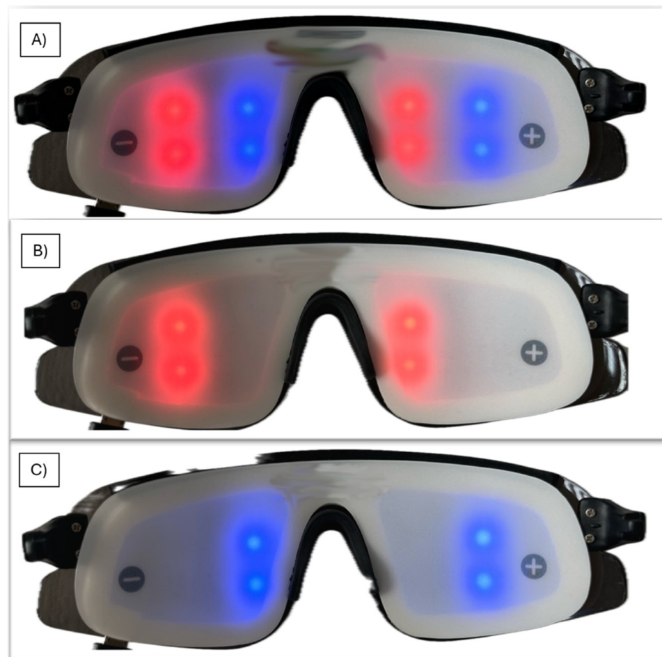
Figure 3. (A) delivering light into both eyes and visual fields. (B) Delivering into right visual field. (C) Delivering into left visual field.
