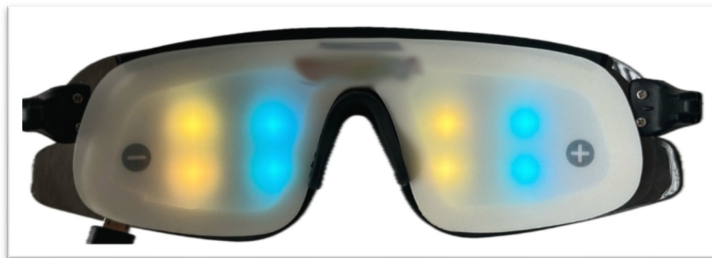
Figure 1. Example of color presentation through a commercial audiovisual entrainment (AVE) device. The device consists of eight light-emitting diodes (LEDs), with four LEDs positioned for each eye. For each eye, two LEDs target the left visual field and two LEDs target the right visual field. In this configuration, the left visual field is illuminated with yellow light, and the right visual field is illuminated with blue light. The colors shown are representative of a common experimental setup; yellow and blue were selected because different wavelengths can evoke distinct physiological and psychological responses, as reported in prior research [44–46].
