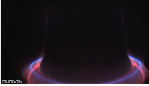
Fig. 1. Visible camera image of a discharge with an XPR (AUG #40007, 3.4 s) seen in blue light emitted by nitrogen, dominated by N^{2+} . Magenta is the typical Balmer emission from deuterium in a divertor leg. (For interpretation of the references to colour in this figure legend, the reader is referred to the web version of this article.)
