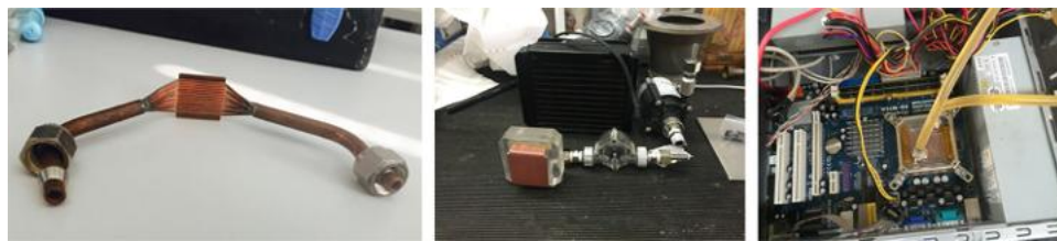
Fig. 49 Micro-channel tested prototype (left) and its application as a heat sink of a computer CPU (center and right)
