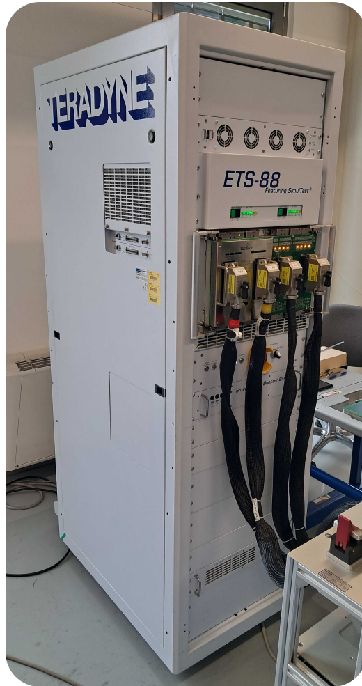
Figure 1.2: Teradyne ETS-88, highly versatile automatic test equipment widely used for the automatic testing of semiconductor devices
