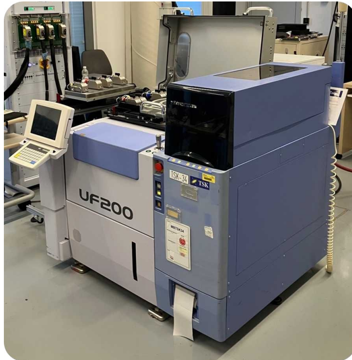
Figure 1.4: Accretech UF200, fully-automatic wafer prober specialised for productive environments
