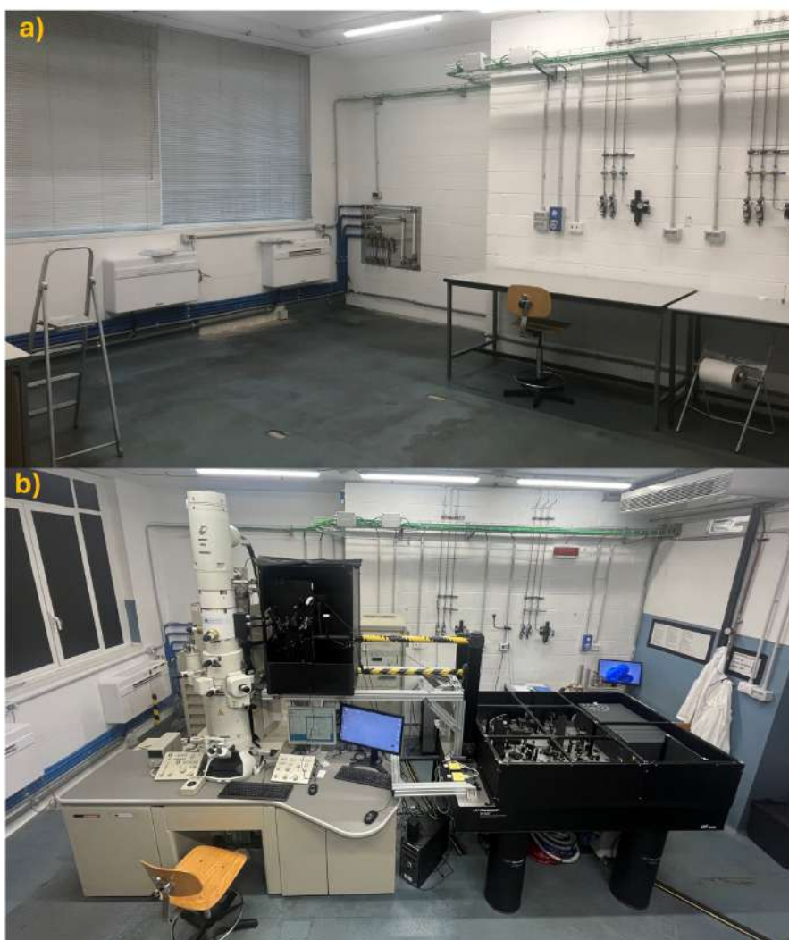
Figure 3.5: a) Laboratory room before the installation of the UTEM setup, at the start of my Ph.D. b) Large view of the complete UTEM setup at UniMiB. The femtosecond laser system (right) is optically coupled to the modified transmission electron microscope (left) via a custom-designed routing system including periscopes and breadboards.
