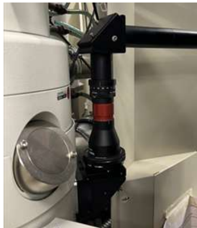
Figure 3.4: Photograph of the optical access implemented at the sample plane in the UTEM setup. The pump beam is injected through the EDX port using a periscope and beam-shaping optics.
