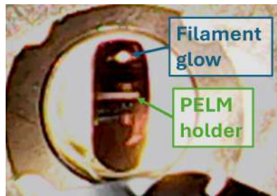
Figure 3.19: Optical camera view of the PELM section through the last dielectric mirror of the UV injection path. The glow from the heated \text{LaB}_6 filament is visible as a reflection on the aluminum UV mirror (top), while the PELM platelet of the holder is seen below it. Because the last dielectric mirror of the UV injection path is transparent in the visible, the camera provides a direct view inside the TEM column, enabling coarse alignment of the UV beam with respect to the cathode.
