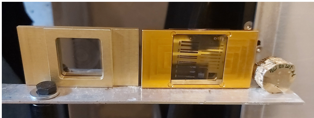
Fig. 5.3 Picture of the Bar pattern and Siemens Star devices used for the experimental evaluation of the spatial resolution of the imaging system.
