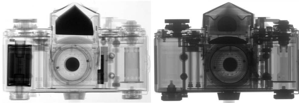
Fig. 1.5 X-rays (left) and neutron (right) radiography of an analogue camera [4]. X-rays are more attenuated by heavier materials, like the metallic parts of the camera, whilst neutrons are more sensitive to light atoms, such as hydrogen, making possible the visualisation of plastic details of the photo apparatus with high contrast.
