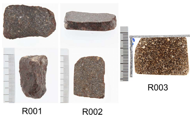
Fig. 2 The three samples from the same meteorite studied in this work: R001 and R002 are bulk samples, whereas R003 is a standard petrological thin section.
