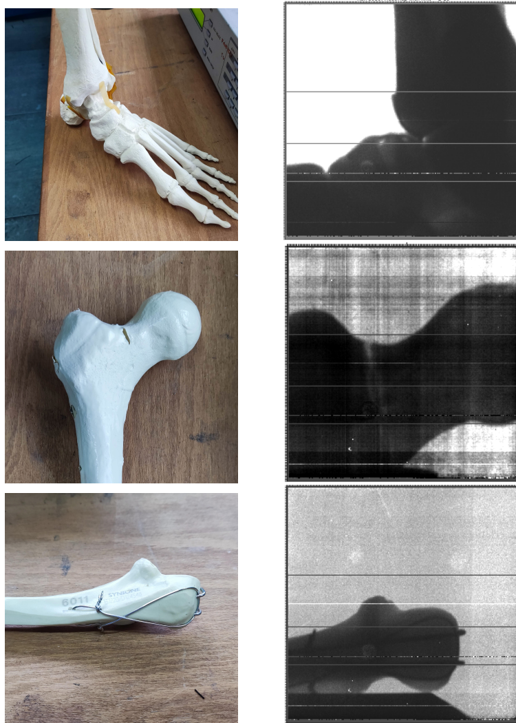
Figure 5. On the left, picture of the observed bone mock-ups. On the right, corresponding images captured with the detector.
