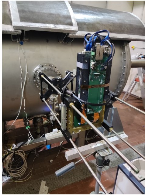
Figure 4.8: Picture of the XR-GEM-1 detector as installed at HVPTF.
