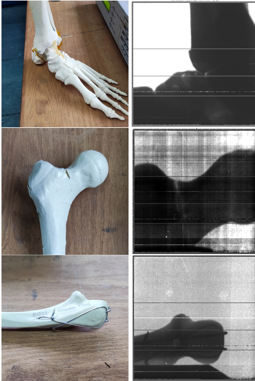
Figure 4.41: On the left, picture of the bone mock-ups used for measurements. On the right, corresponding heatmaps of data captured with the strip GEM detector.
