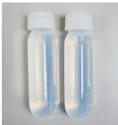
Fig. 2 PFA vials with screw caps. Volume 30 mL, diameter 25 mm, and total height 90 mm
