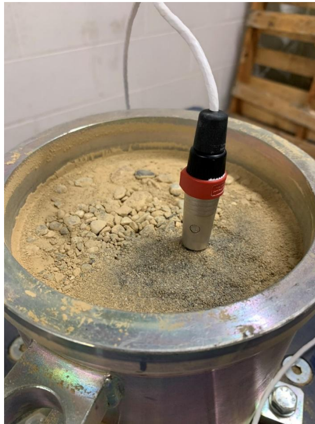
Figure 3.4 – ThermTest’s TLS-100 needle probe while operating a measurement on a remoulded sample in e_{min} conditions.
