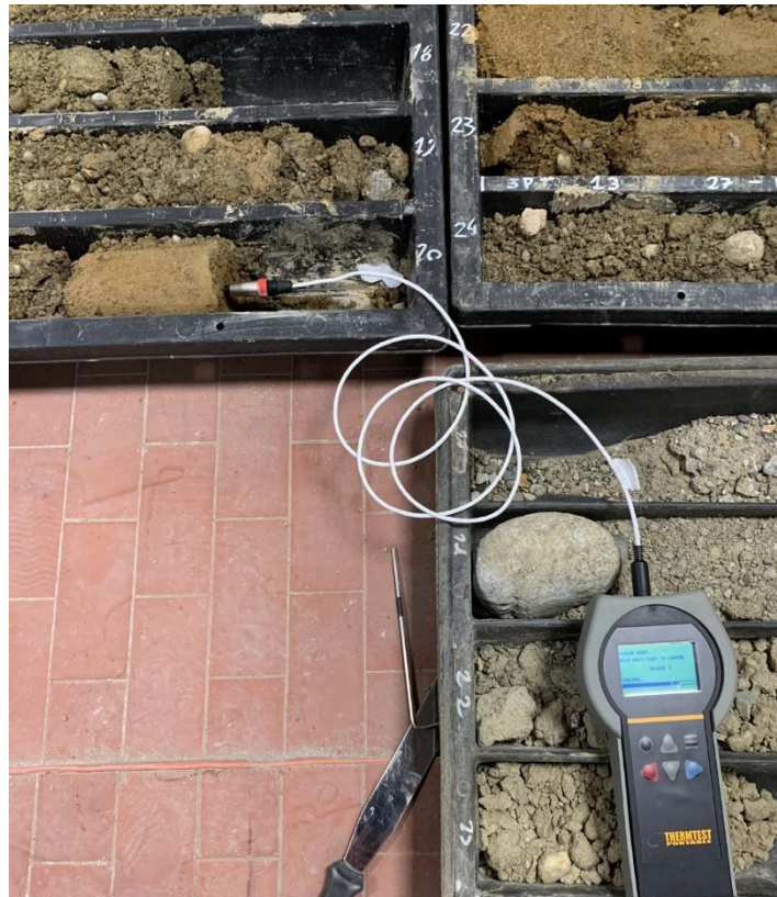
Figure 3.3 - ThermTest's TLS-100 needle probe while operating a measurement on an intact sample.
