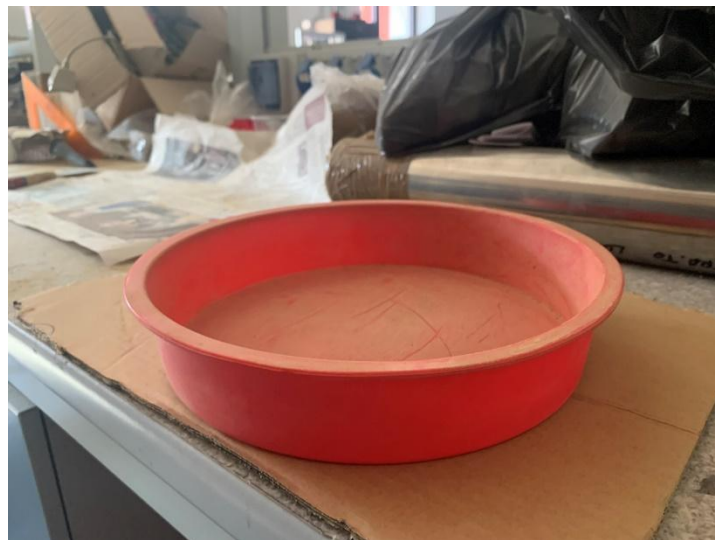
Figure 3.12 - Container selected for conducting the thermal conductivity test.
