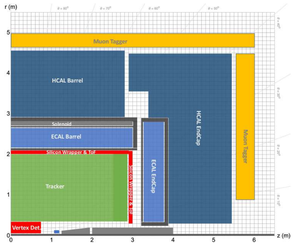
Fig. 94 Longitudinal cross section of the top right quadrant of the ALLEGRO concept detector. The LumiCal, the compensating solenoid, and the final-focus quadrupole are displayed along the z axis
