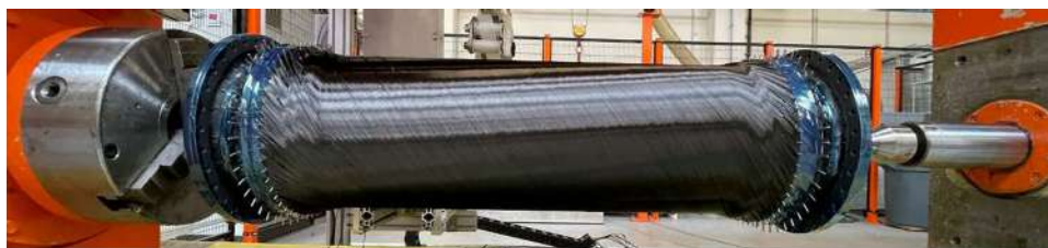
Fig. 117 Full liner-less tank demonstrator, 1 m length, 0.3 m diameter, and 5 mm wall thickness. Manufacturing process: filament wet-winding, non-crossing, out-of-autoclave curing
