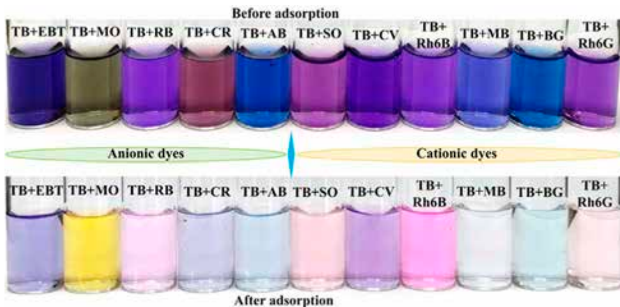
Figure 11. Trypan blue (TB) selectivity with anionic and cationic dyes using NZB LTH.
