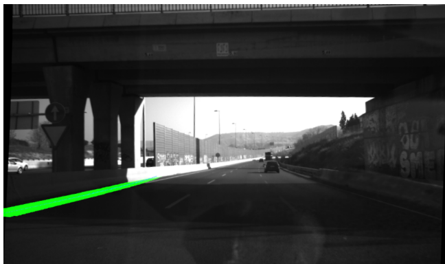
FIGURE 1: The figure illustrates a scenario with high contrast, where our basic line detector faces challenges in identifying a substantial portion of the road markings.
