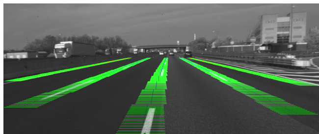
FIGURE 8: An image from the A4 dataset showing an annotated lane change event marked with the Crossing Flag.
