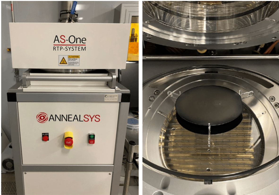
Figure 2.2: Annealsys As-One150 RTP system used in this work (left) and zoom of 4" substrate used as support for diffusion and oxidation on small samples (right).
