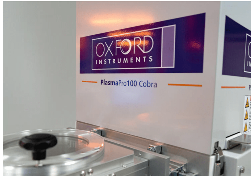
Figure 2.10: RIE instrument installed at the INRIM laboratories.
