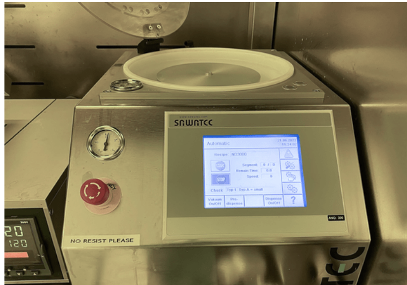
Figure 2.1: SAWATEC SM-150 machine, the spincoater used during this work.
