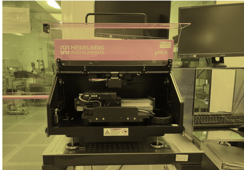
Figure 2.5: Tabletop Maskless Aligner \mu MLA used for photolithography.
