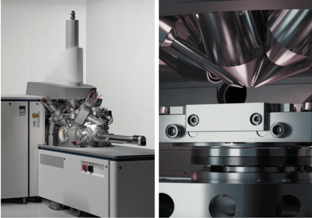
Figure 2.14: M6 IONTOF apparatus used for ToF-SIMS analysis.
