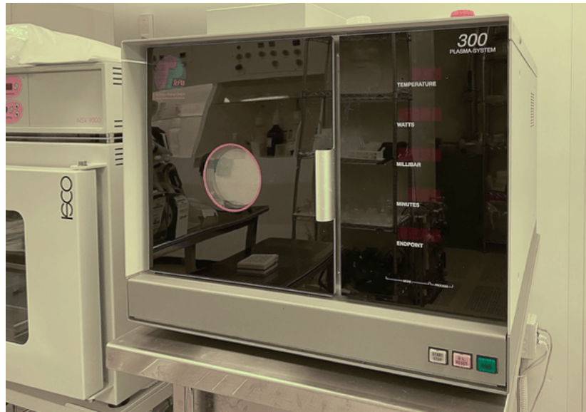
Figure 2.3: Technics Plasma 300 machine, used for plasma cleaning processes.
