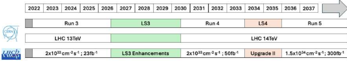
Figure 1.2: Timeline of the LHC and LHCb experiment. Although the HL-LHC will start operation in 2030, the luminosity in the LHCb experiment will not be increased until LHC Run 5. LHCb Upgrade II will be installed during LS4, while some sub-detectors will introduce some enhancements already during LS3. Edited from [26].
