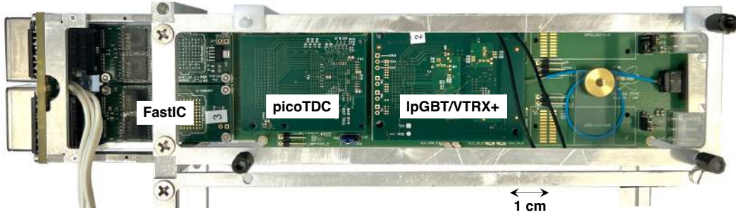
Figure 1.29: Second prototype of optoelectronic readout chain consisting of a carrier board with (from left to right) the photon sensor board, FastIC ASIC plugins, picoTDC plugin and optical link plugin.
