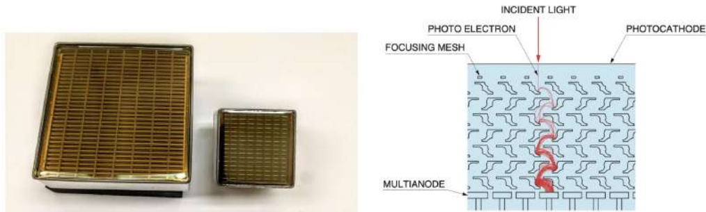
Figure 1.21: Left: the MAPMTs used in LHC Run 3 RICH detectors with the 2-inch model on the left and the 1-inch model on the right. Right: scheme of the internal structure of the MAPMT [38].
