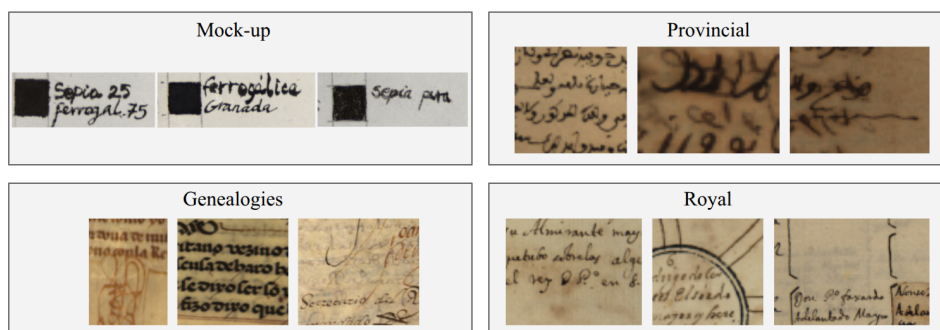
Figure 1. Sample fragments used within this study, visualized in false RGB colors from the VNIR range (630, 535 and 430 nm bands).
